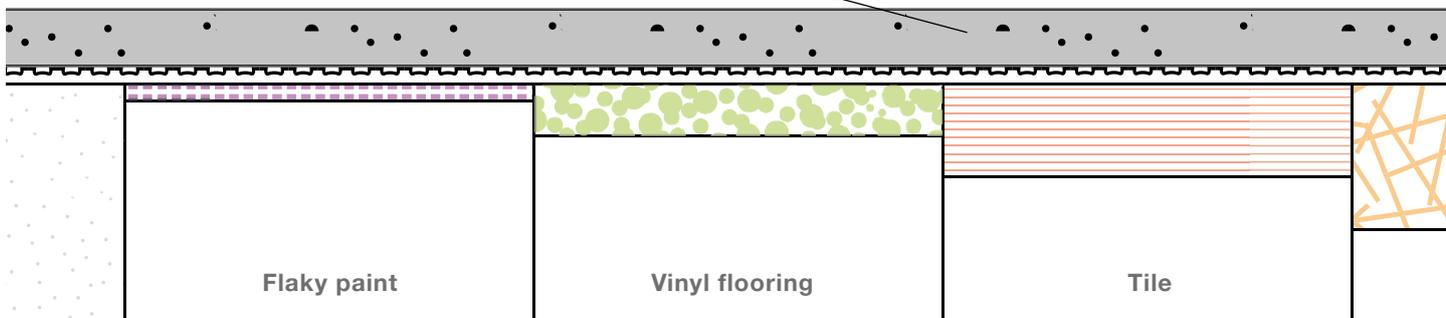
Altro Cantata allows a quick fit without compromising on performance. It features a studded surface on the underside of the floor. This unique formulation allows the floor to lie flat and perform like a traditional adhered floor without the need for an adhesive.
